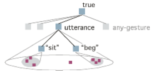
Figure 2: In our work the state space is represented by a percept tree. The percept tree maintains a hierarchical representation of the sensory input where leaf nodes represent the highest degree of specialization and the root node matches any sensory input. The structure of the tree is sequentially discovered and refined with time as indicated by its utility with respect to getting reward.
